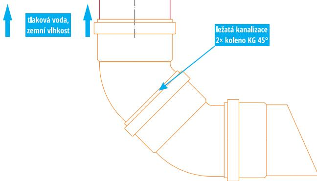
TVAROVKA JE SOUČÁSTÍ ROZVODU ODPADNÍ/DEŠŤOVÉ KANALIZACE – SYSTÉM KG/KG 2000
